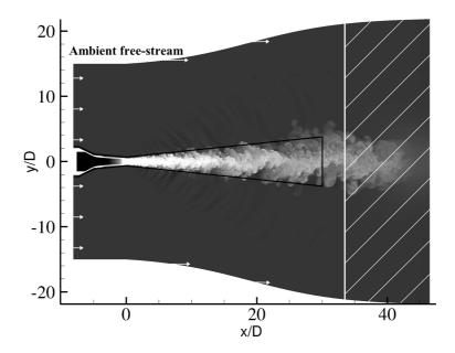
Figure 1: View of the computational domain (cutting plane z = 0) with a density field from S3. The black line represents a typical location of the FWH surface (see details further). The hatched region, starting at the vertical white line, corresponds to the part of the domain where a sponge treatment is applied.
