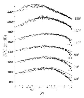
Figure 10: Comparisons of far-field sound narrowband spectra between numerical results from simulations S2 (—) and S3 (----) and experimental data (……). Spectra are calculated every 20° from 50° (upstream) to 150° (downstream). Numerical and experimental spectra are staggered as in Fig. 8.
