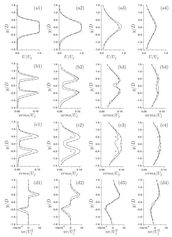
Figure 6: Comparisons between numerical results from S2 (----), S3 (---) and experimental data (---). Radial profiles of time-averaged streamwise velocity (a row), RMS of streamwise (b row) and radial (c row) velocity components and turbulent shear stress uv (d row) for x/D = 2.5, 5, 10, 15 (columns 1 to 4), at z = 0. Experimental RMS data calculated from the integration of velocity spectra displayed in section V.C are displayed by +.
