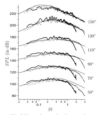
Figure 14: Comparisons of far-field sound narrowband spectra between experimental measurements (.....) and numerical results from simulations S2 (....) and S2c (....), from 50° (upstream) to 150° (downstream). Numerical and experimental spectra are staggered by adding a cumulative shift of 20 dB for each angle (100 dB are added for angle 150°). For sake of legibility, spectra of the S2c case are shown up to St = 2 to avoid mixing staggered graphs at different angles.
