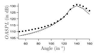
Figure 11: Comparisons of far-field overall sound pressure level at 100 D between numerical results from S2 (—) and S3 (----) and experimental data (symbols).
