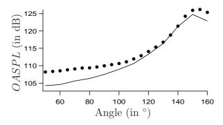
Figure 9: Comparisons of far-field overall sound pressure level at 100 D between numerical results from S1 (—) and experimental data (symbols).
