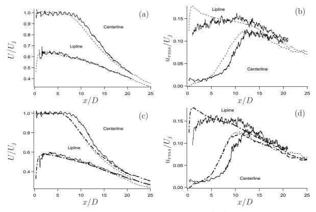
Figure 4: Comparisons between numerical and experimental (—) results along the centerline and a lip line between x = 0 and x = 25 D. Time-averaged (a) and RMS (b) of streamwise velocity for the unheated case S1 (----), time-averaged (c) and RMS (d) of streamwise velocity for the heated cases S2 (----) and S3 (---).
