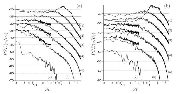
Figure 7: Comparisons between numerical (—) and experimental (—) narrowband power spectral density of streamwise (a) and radial (b) velocity for simulations S3 along the lip line at x = 0.5 D (1), x = 1.25 D (2), x = 2.5 D (3), x = 5 D (4), x = 10 D (5), x = 15 D (6), x = 30 D (7). A cumulative shift of -5 dB has been added to the PSDs to separate the plots, from -5 dB at x = 1.25 D (2) to -30 dB at x = 30 D (7).
