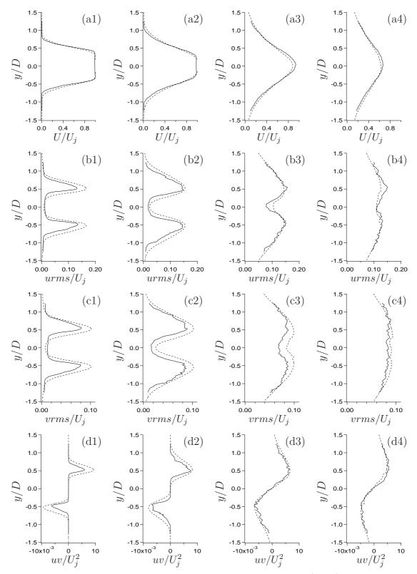
Figure 5: Comparisons between numerical results from S1 (----) and experimental data (---). Radial profiles of time-averaged streamwise velocity (a row), RMS of streamwise (b row) and radial (c row) velocity components and turbulent shear stress uv (d row) for x/D = 2.5, 5, 10, 15 (columns 1 to 4), at z = 0.
