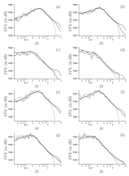
Figure 12: Near-field sound pressure levels at r = 3D (a-d) and r = 5D (e-h). Comparison of numerical results directly extracted from simulation S3 (----), using S3 and FWH integration (—) and experimental measurements (……) at r = 3D and x = 10.7D (a), x = 13.7D (b), x = 16.7D (c), x = 19.7D (d) and at at r = 5D and x = 13.15D (e), x = 16.15D (f), x = 19.15D (g), x = 22.15D (h). Numerical results have been empirically shifted in the axial direction by +4D.
