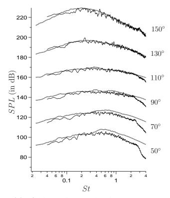
Figure 8: Comparisons of far-field sound narrowband spectra at 100 D between numerical results from S1 (—) and experimental data (……). Spectra are calculated every 20° from 50° (upstream) to 150° (downstream). Numerical and experimental spectra are staggered by adding a cumulative shift of 20 dB for each angle (100 dB are added for angle 150°).
