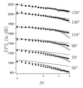
Figure 15: Comparisons of far-field high-frequency sound between experiment (......) and numerical results from simulations S2 ( $\circ$ ), S3 ( $\bullet$ ) and S2r (+), from 50° (upstream) to 150° (downstream). Numerical and experimental spectra are staggered by adding a cumulative shift of 20 dB for each angle (100 dB are added for angle 150°). Narrowband spectra from simulations are displayed with symbols, every St=0.12 to be able to differentiate the results.
