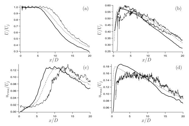
Figure 13: Comparisons between numerical results from S2 (----) and S2c (----) and experimental data (----) along the centerline (a,c) and a lip line (b,d), between x = 0 and x = 20 D: time-averaged (a,b) and RMS (c,d) of streamwise velocity. Experimental data along the lip line are measured along y = 0.5 D and y = -0.5 D and both displayed (b,d) using a solid line.
