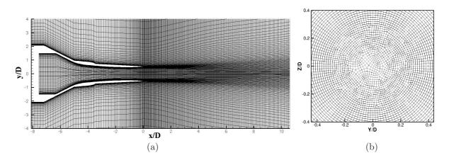
Figure 2: Grid used for the LES in cases S1 and S2. (a): Cutting plane z = 0 through the center of the nozzle. Every second grid point is shown in both directions. (b): Cross section of the grid used for cases S1 and S2, at location x/D = 10.
