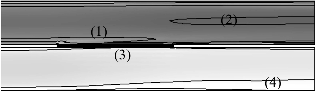
Figure 11. Field and isolines of time-averaged streamwise velocity over the cutting plane z = 0 using model UM2. Scale is the same as for Fig. 10. Zoom on the section between 120 d < x < 288 d .
