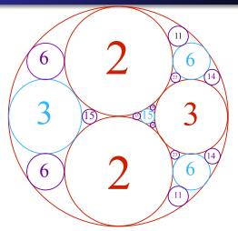
Each circle is labeled with its curvature :  $curv(C) = \frac{1}{radius(C)}$ The curvature of the exterior circle is -1 (oriented to the exterior so interiors are dijoints).
