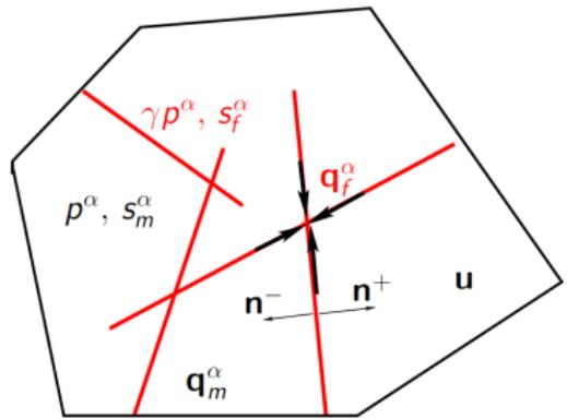
Following [Coussy], the *equivalent pressures*  $p_m^E$  and  $p_f^E$  are based on the **capillary energy density**  $U_{rt}(p_c) = \int_0^{p_c} q (S_{rt}^{\text{nw}})'(q) dq$ , rt = m, f and
