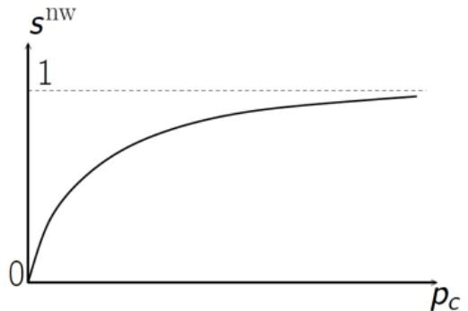
$$\begin{cases} \partial_t(\phi S^\alpha(p_c)) + \operatorname{div}(\mathbf{q}^\alpha) = 0, & \alpha = \text{nw}, \text{w}, \\ p_c = p^{\text{nw}} - p^{\text{w}} \end{cases}$$
