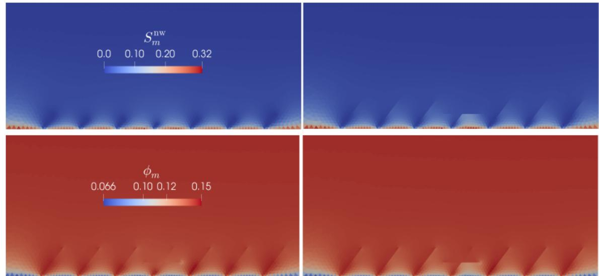
Gas saturation (top) and porosity (bottom) given by the continuous (left) and discontinuous (right) models
