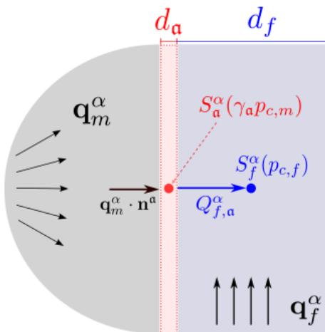
$$Q_{f,a}^\alpha \approx \eta_a^\alpha(S_a^\alpha(\gamma_a p_{c,m}))K_{f,n}\left(\frac{\gamma_a p_m^\alpha - p_f^\alpha}{\frac{d_f}{2}} - \rho^\alpha \mathbf{g} \cdot \mathbf{n}^a\right)^+$$
