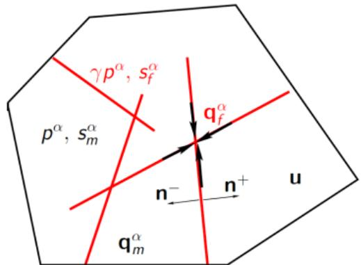
Fracture model with **no contact**:  $\boldsymbol{\sigma}^T(\mathbf{u})\mathbf{n}^\pm = -p_f^E \mathbf{n}^\pm$ ,
