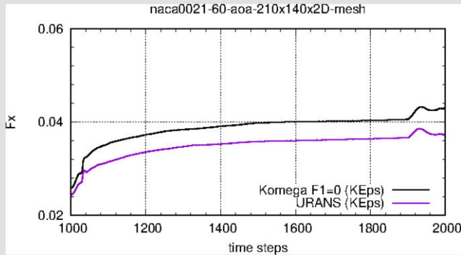
Validation step 2: set  $\phi = 1$  to recover  $k-\omega$  solution:
