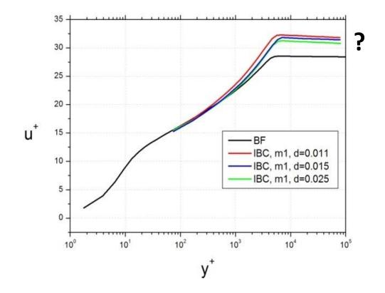
IBC, m1 – immersed boundary method with WF using coarse mesh m1 with near-wall dy = 1e-02 BF – body-fitted approach with No-Slip using mesh with near-wall dy = 1e-05
