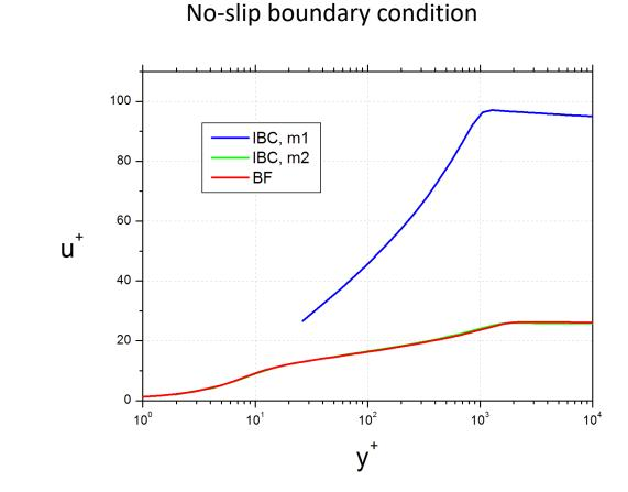
IBC, m1 – immersed boundary method using coarse mesh m1 with near-wall dy = 1e-02
