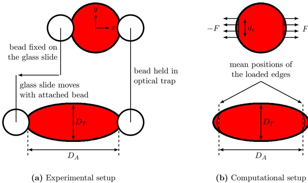
**Fig. 1** (a) Illustration of the experimental setup of Mills et al. (2004). The axial ( $D_A$ ) and transverse ( $D_T$ ) diameters of the stretched RBC are measured. (b) Computational setup used to simulate the optical tweezers experiment. A stretching force  $F$  is applied over the two circular edges delimitating the contact areas between the RBC and the beads, with a contact size  $d_c = 2 \mu\text{m}$ .
