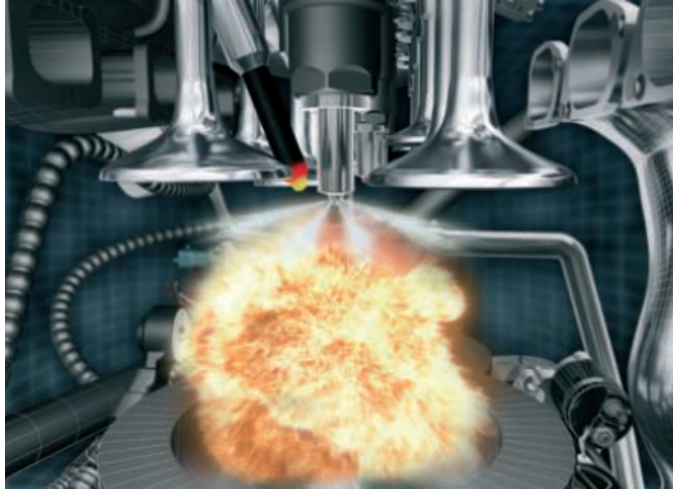
Figure 1: Artistic image of an IC engine combustion chamber. It illustrates the complexity of the flows : sprays atomization, multi-phases flows, combustions, wall-bounded flows
