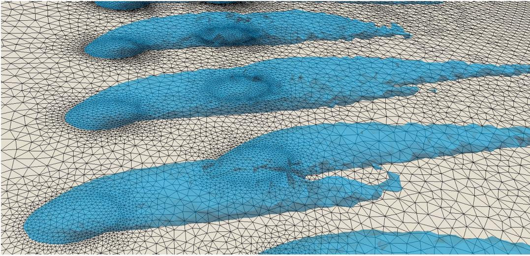
Figure 5.8: Isosurface of the coolant jet allowing to visualize the boundary mesh in the modeled case. Extrated from [79]
