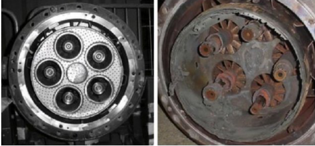
Figure 1.2: Burner nozzle without (left) and with (right) damage due to combustion instabilities. From [1].
