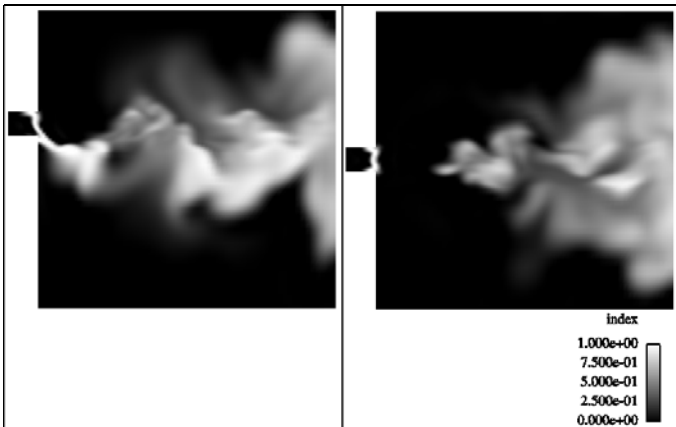
Figure 19 – Mixing index visualization at T_0+28ms for the first configuration. Symmetry plane (left) and horizontal plane (right)
