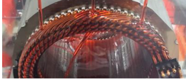
Figure 1.3: Oil injection experiments on end-winding [27]
