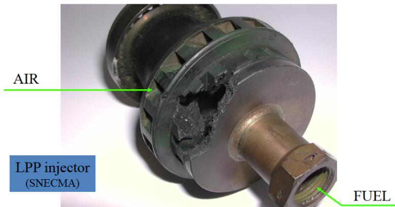
FIGURE 1.7: The injector of an LPP design jet combustor, after a combustion instability.
