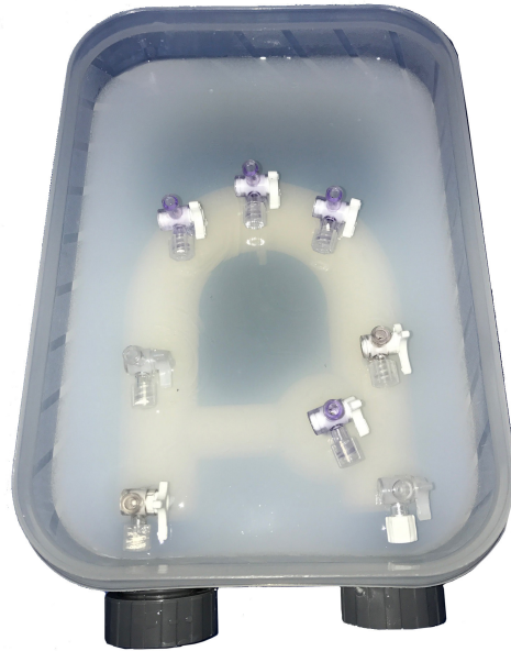
Figure 4.2: a). (left) Engineering drawing and (right) the first version of the flow phantom, made with photopolymer resin. b). (left) Second version of the phantom, made with Nylon, and (right) immersed within the silicon bath .
