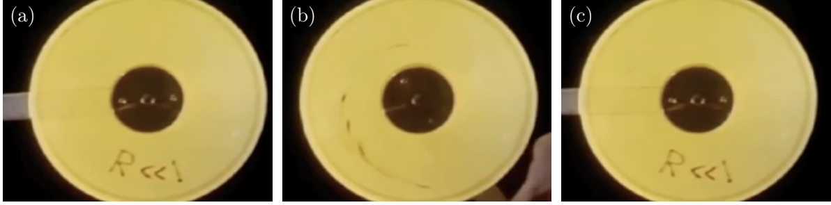
Figure 2.1: Reversibility of Stokes flow visualized by G.I. Taylor [Taylor 1967]. (a) A text is written with dye deposited on a viscous fluid in a cylindrical tank. (b) The outer wall is rotated for one and a half turn in the clockwise direction, resulting in the deformation of the dyed text. (c) Rotating the outer cylinder counter-clockwise back to its initial position also brings back the dye to the initial writing according to the reversibility principle.
