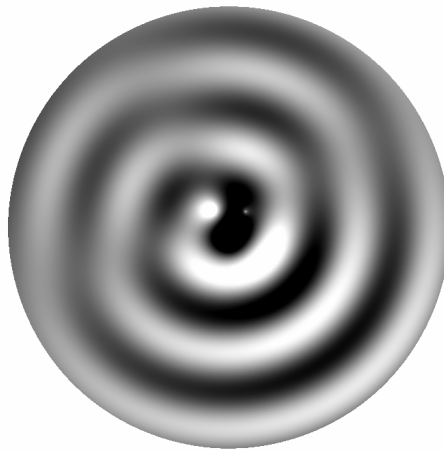
Figure 4.9: Acoustic field produced by three monopoles out of phase. p' = |\hat{p}| \cos(arg(\hat{p}))
