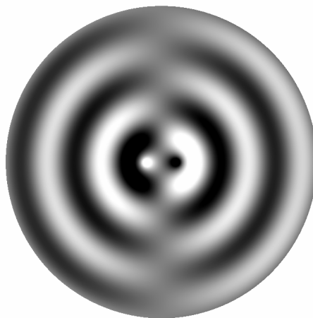
Figure 4.6: Acoustic field produced by a dipole. p' = |\hat{p}| \cos(\arg(\hat{p}))
