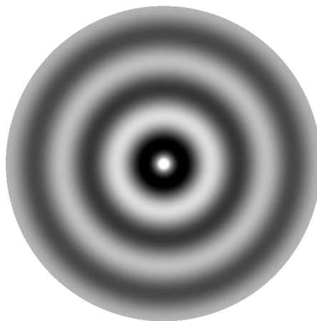
Figure 4.3: Acoustic field produced by a monopole. p' = |\hat{p}| \cos(\arg(\hat{p}))
