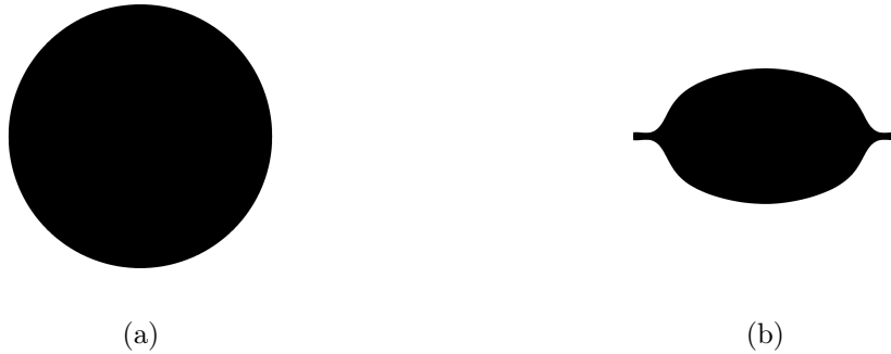
Figure 3.13: Images of the cross-sectional areas of the inlet (a) and valve (b) used to calculate the effective opening area (EOA).
