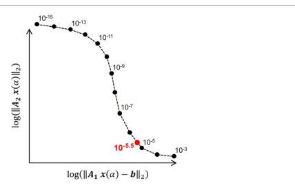
**Figure 5.** Automatic selection of the regularization scalar: an L-curve is plotted from a set of regularization parameters (black dots). We choose the regularization parameter that provides the rising point of inflection (here  $10^{-5.5}$ , red dot). This example is from a patient at the end of early filling. In practice, we used five  $\alpha$  values to generate an L-curve by fitting an hyperbolic tangent function.
