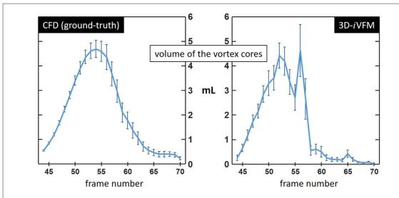
**Figure 9.** *In silico* results: vortex volumes derived by 3D-iVFM versus actual CFD velocities. The vortical regions were detected by using the *Q*-criterion. A voxel belonged to a vortex if its *Q*-value was greater than a threshold. Several thresholds were used: the error bars illustrate the standard errors of the means (SEM).
