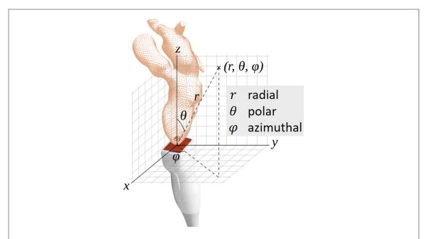
Figure 3. The data and equations that are included in 3D-iVFM (intraventricular Vector Flow Mapping) are expressed in this spherical coordinate system.
