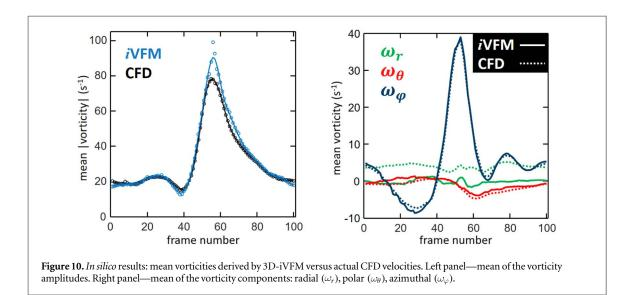
prominent (figure 10, right) compared with the radial ( $\omega_r$ ) and polar ( $\omega_\theta$ ) components. 3D-*i*VFM produced vorticity profiles consistent with those given by CFD (ground-truth).
