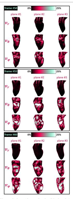
**Figure 8.** *In silico* results: maps of the normalized errors. The rows refer to the radial, polar, and azimuthal velocity components, respectively. The columns refer to the three planes similar to those of the triplane mode. The frames #50, #55, and #60, occurred during early filling (see figure 6).
