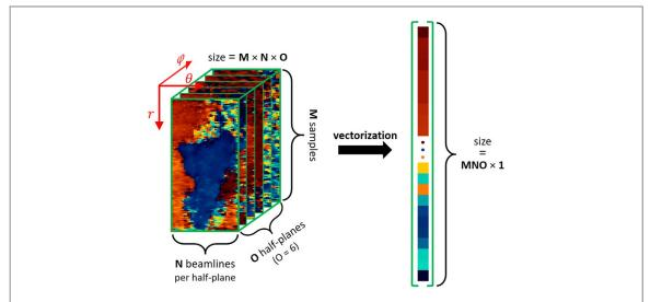
**Figure 4.** The 3D-iVFM was derived using a 3rd-order tensor formalism. The equations were then vectorized to obtain a sparse symmetric linear system. The dimensions of the tensors were related to the coordinates  $(r, \theta, \varphi)$  of the spherical system.
